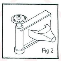
4. To have the Driving Rubber Cam connect with outer rim of workpiece, so that the workpiece will be rotate properly in tune with the rotation of the cam, it is correctly for adjustment, connection can not be too tight or loose, adjusting control gage of product length.
